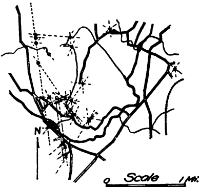
FIG. 200. — Fissure springs arranged upon lines of rock fracture at intersections, Pomperaug valley, Connecticut.
